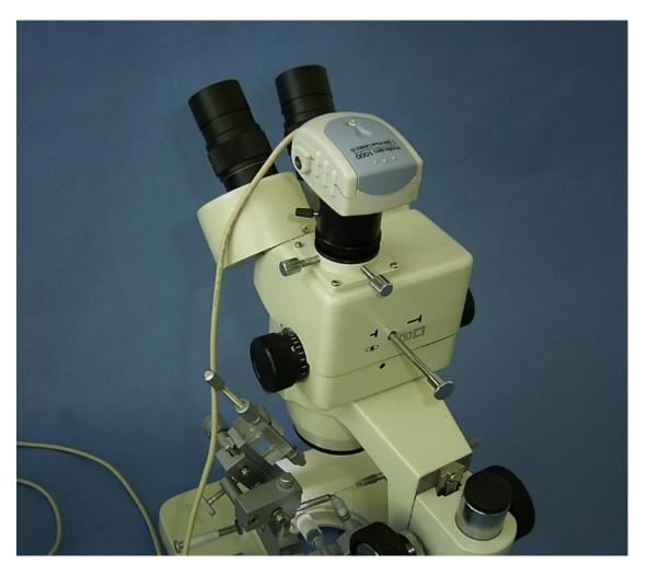
**Stereomicroscop SMZ Zoom 143 with Camera Moticam 1000** The connection between camera and optics is made with CCD adapter 0,5x, which is provided as accessories to the microscoope. **Art.-No. 2.10**
