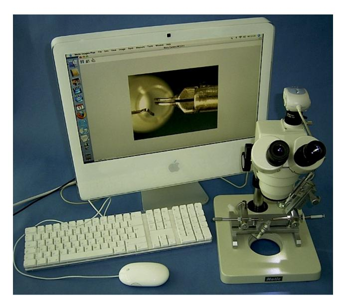
**Stereomicroscop SMZ Zoom 143 with Moticam 1000** Attached is the Apple-computer iMac. On the screen the pressure grip forceps is shown. Under the optics is the instrument 1.02.
