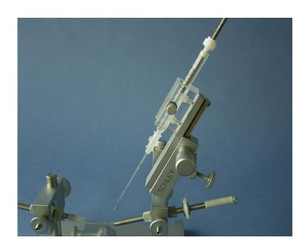
The cylinders directly on the device without hose. The Lueradapter (2 x female) connects the glass tip with syringe.
